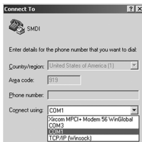
Figure 14-8. HyperTerminal Connect Port Selection
