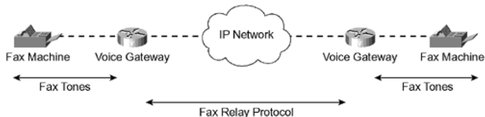
Figure 8-4. Fax Relay Over an IP Network
